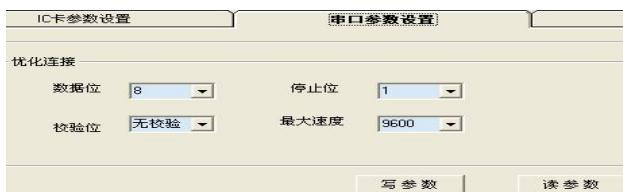
This screenshot shows the 'Serial Port Parameter Settings' section of a software interface. It includes fields for 'Data Bits' (set to 8), 'Stop Bits' (set to 1), 'Parity' (set to 'No Parity'), and 'Baud Rate' (set to 9600). At the bottom are 'Write Parameters' and 'Read Parameters' buttons.
